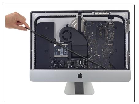
Remove the lower support bracket (a.k.a. "chin strap") from the iMac enclosure.
