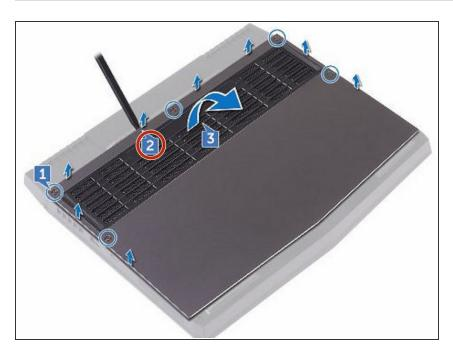
Using a plastic scribe, gently pry the base cover to release the tabs on the base cover from the slots on the computer base.
