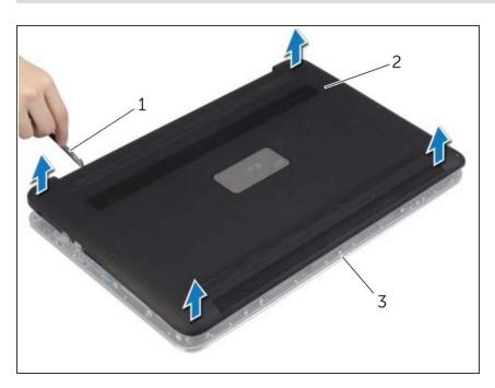
Using a spudger or some other prying tool (#1), pry off the basecover assembly from the rest of the system.
