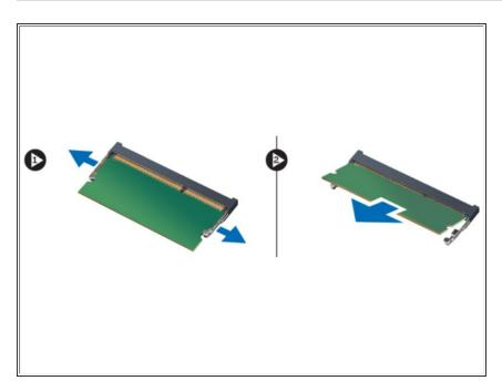
Use your fingertips to spread apart the securing clips on each end of the memory module connector until the memory module pops up and remove the memory module from its connector on the system board by drawing the module from the system board at 45-degree angle.
