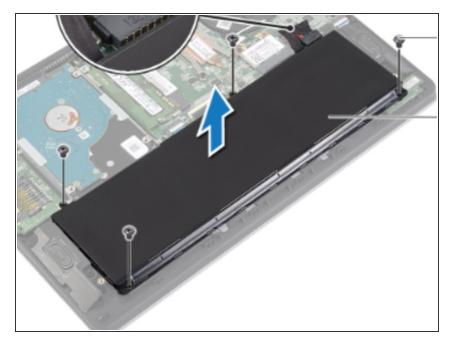
Align the screw holes on the battery with the screw holes on the palmrest assembly and place the battery on the palm-rest assembly.
