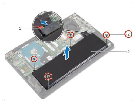
Remove the screws that secure the battery to the palm-rest assembly.
