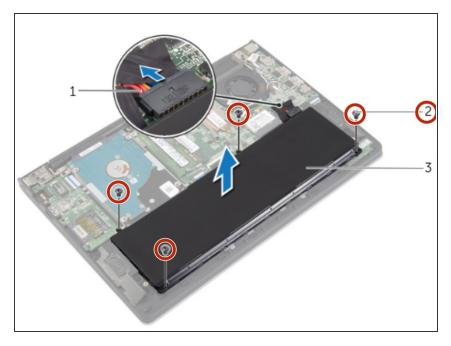
Replace the screws that secure the battery to the palm-rest assembly.
