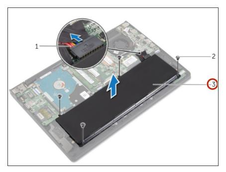
Lift the battery, along with its cable, off the palm-rest assembly.
