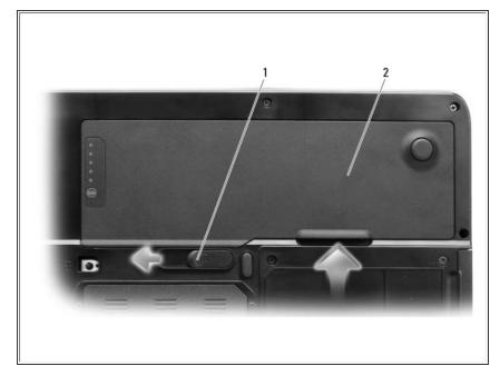
Slide and hold the battery-bay latch release on the bottom of the computer, and then lift the battery from the bay.
