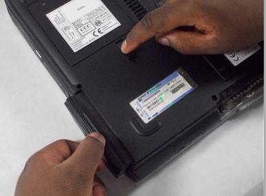
• While still holding the switch up, remove the battery.
