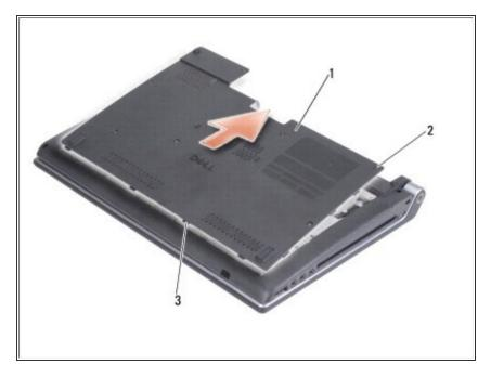
Loosen the seven captive screws on the base cover and lift the cover off the computer at an angle as shown in the figure.
