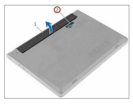
Slide the battery-release latch to the unlocked position.
