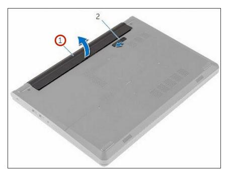
Place **NEW** the battery in the battery bay and snap the battery into place.
