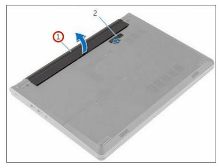
Lift the battery at an angle and remove it from the battery bay.
