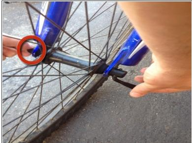
• Find the quick release lever on the outside of the bike's fork on the right hand side. Turn the level counter clockwise loosening the lever until it comes off.
