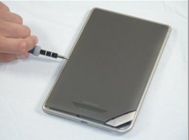
Slide the spudger around the edges of the Nook to loosen the back panel.
