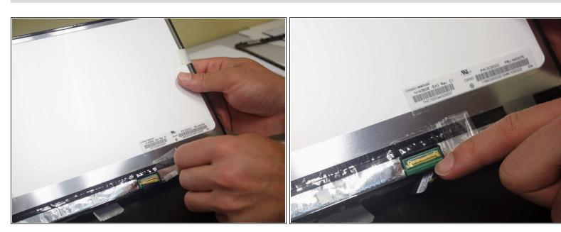
Remove the connector located at the bottom of the back of the screen.
