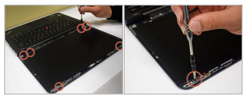
Take off the 6 screws using the Philips head #1.
