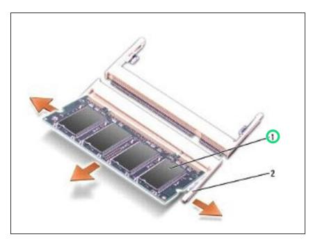
Slide the **NEW** module firmly into the slot at a 45-degree angle, and lower the module until it clicks into place. If you do not feel the click, remove the module and reinstall it.
