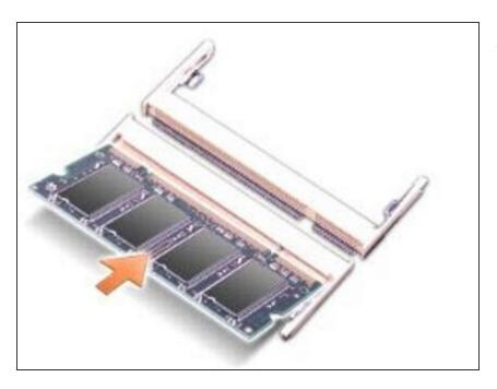
Align the notch in the module edge connector with the tab in the connector slot.
