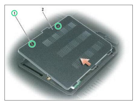
Loosen the two captive screws on the memory module/modem cover and remove the cover.
