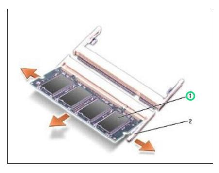
Remove the module from the connector at a 45-degree angle.
