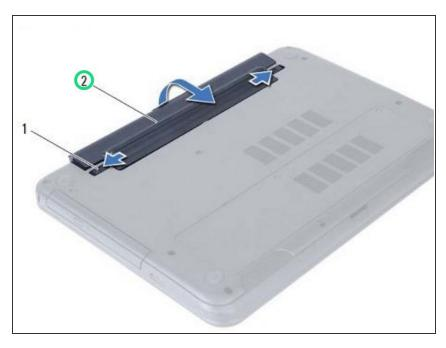
Lift and remove the battery off the computer base to disconnect it from the computer.
