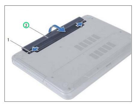
Align the tabs on the **NEW** battery with the slots on the battery bay and snap the battery into place.
