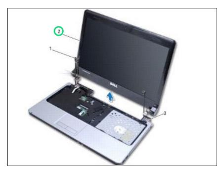
Hold the display while you remove the three screws that secure the display assembly to the computer base.
