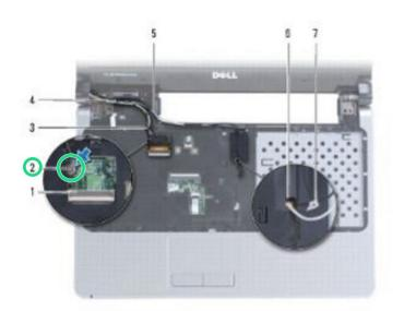
Disconnect the display cable and remove the screw from the system board.
