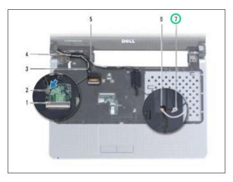
Route the antenna cables through the slot in the computer base.
