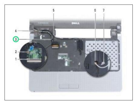
Note the routing of all the cables and remove them from their routing guides.
