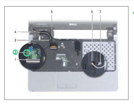
Replace the screw and connect the display cable.
