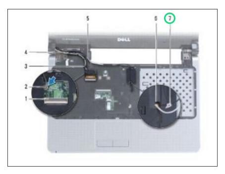
Pull the Mini-Card antenna cables up through the slot in the computer base.
