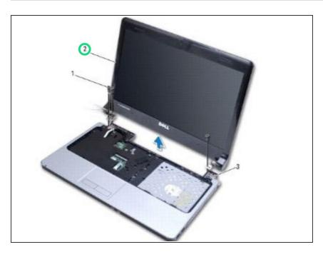
Using the alignment posts, place the display assembly in position and replace the three screws that secure the display assembly to the computer base.
