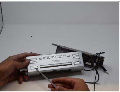
Gently use a flat head screwdriver in the gaps between the button and device body to loosen them from their positions.
