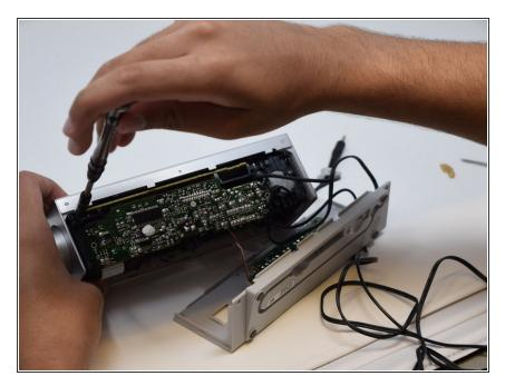
Using a small tool, push the buttons outward by pressing on them firmly until they pop out of their place.
