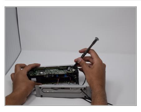
Insert the new button from the inside of the device, pushing it towards the front with gentle force until it locks into place.
