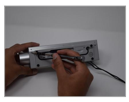
Remove the back cover of the device by unscrewing all screws and prying it open.
