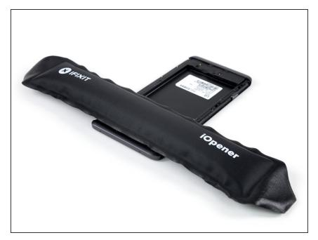
Use an iOpener to loosen the adhesive beneath the rear lens cover.
