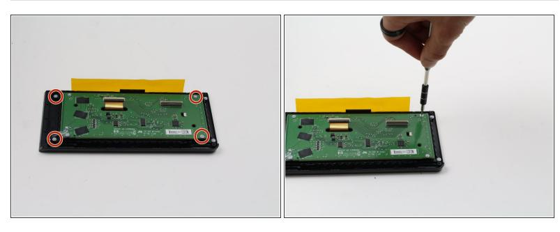
Remove the four 4.8 mm T6 screws from the back of the display motherboard.
