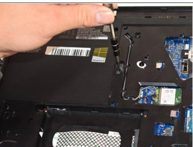
Remove one 6mm Phillips #0 screw holding in the optical drive.
