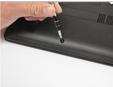
Remove the three 6mm Phillips #0 screws holding the back access panel on.
