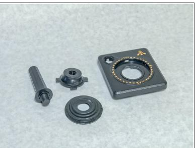
• The joystick will now unscrew (counter-clockwise) and you can disassemble the top of the controller into these four parts.
