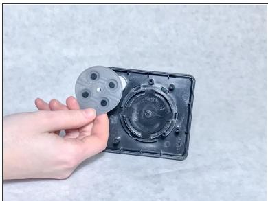
Remove the rubber pad from the joystick.
