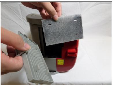
Remove the used filter from the device.
