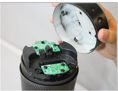
Firm grip the bottom and wiggle upwards to remove bottom.
