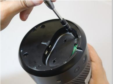
Use a #10 Torx screwdriver to remove four 14 mm screws.
