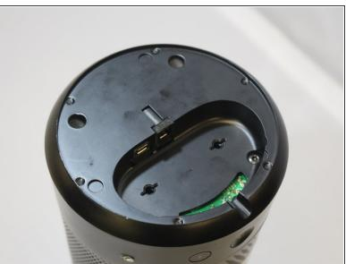
Use a metal spudger to remove rubber bottom.
