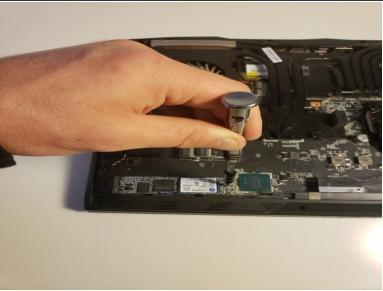
Remove the single 1.2mm screw securing the video card to the laptop using the JIS #0 screwdriver.
