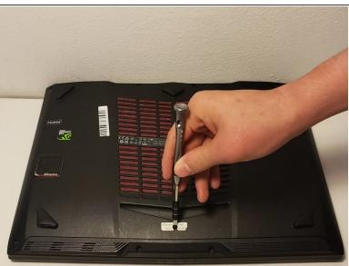
Remove the six 1.2mm screws on the bottom plate of the laptop using a JIS #0 screwdriver.
