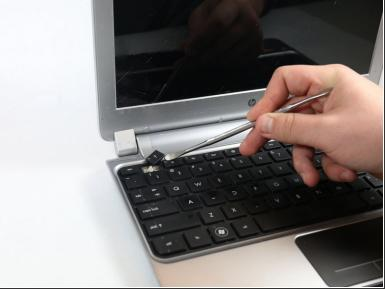
Softly place the tool about an eighth of an inch under the key, and gently pry the key off by lifting upwards. To reassemble your device, follow these instructions in reverse order.
