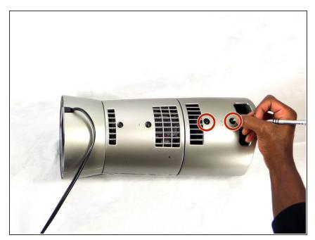
On the backside of the fan, remove the top two 4mm Phillips #Y1 screws using PH 1 bit and Magnetic Driver
