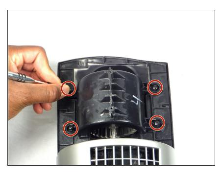
Remove all four 4mm screws using the Phillips #1 screwdriver.
