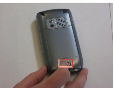
Remove the battery cover by pressing on the small rectangular button located on the back of the phone.
