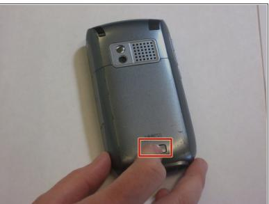
Remove the battery cover by pressing on the small rectangular button located on the back of the phone.
