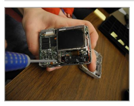
Unscrew the right metal bracket of the viewing lens
