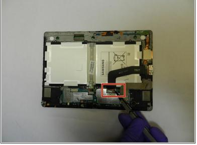
• After taking off the back cover, use a pair of tweezers to disconnect the two (T807) ribbons.
