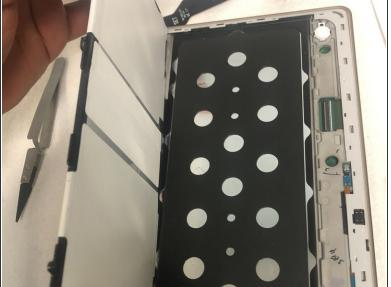
Remove the battery using a spudger.
