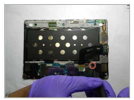
Use a Phillips #00 screwdriver to remove the screw holding the motherboard.
