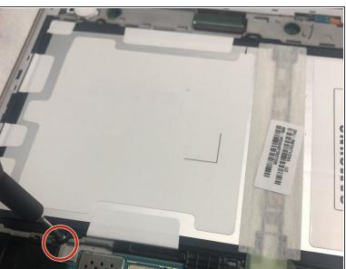
Remove the four screws holding down the battery using the Phillips #000 screwdriver.
