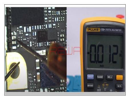
Next, let's continue with the signal amplifier power supply voltage, VPA\_APT. Measure the voltage value of corresponding capacitor, C4108. There is no voltage value. Normal voltage value should be 3V7.
