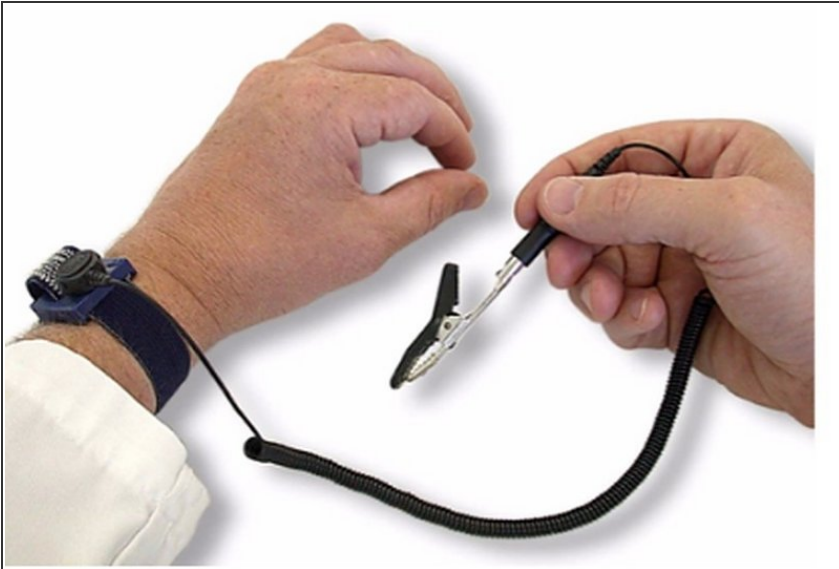
Figure A-4. ESD band and cable
