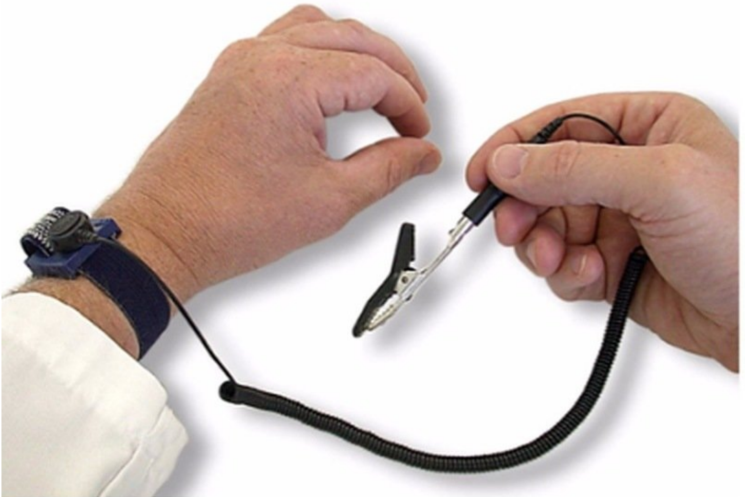
Figure A-4. ESD band and cable
