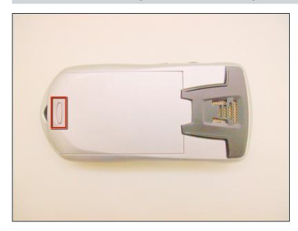
With the back of the device facing you, press down on the button while sliding the battery casing away from the speaker to remove it.
