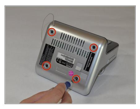
Unscrew the four 15.5 mm Phillips #2 screws that hold the bottom panel to the dock.
