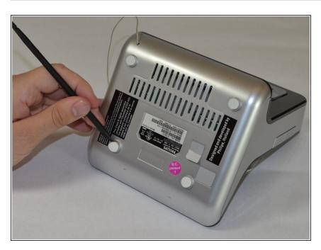
Pry off the four white feet with the pointed end of the spudger
