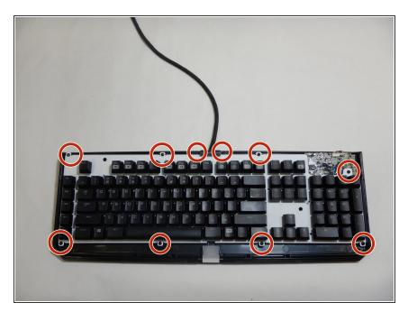
Using a Phillips #1 screwdriver, remove all ten screws found along the outer edges of the keyboard.
