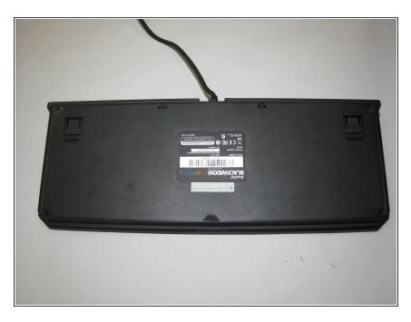
Insert the Jimmy along the edges of the back panel and remove the back panel from the device.
