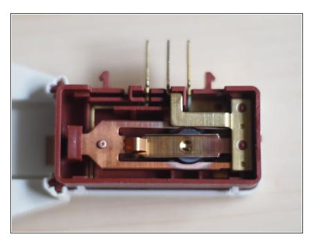
• Remove the door interlock from your device. On my washing machine I had to remove the rubber-lid and loosen two screws. Than the interlock came of with a 3-pol cable attached. On the backside was a plastic plate which had to be unscrewed, too.
