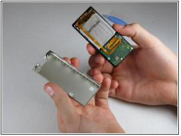
Work your way around the Zune until the back cover comes free. Remove the back plate and set it aside.
