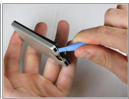
Insert the Zune opening tool between the faceplate and the back cover, starting from the top and slowly work your way around the device.
