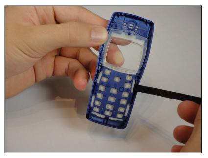
Using the flat end of the spudger, push out the 4 rubber tabs on the back of the keypad to remove it.
