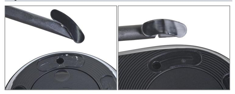
• Repeat the procedure to remove the two remaining lower mouse feet.
