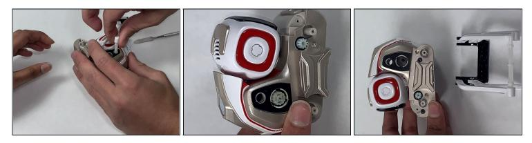
Remove the long white spring that is attached to the right short arm from the center of the body using your hands and fingers to pull it out.
