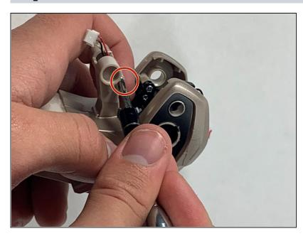
Remove the 7.5 mm screw from the gold bar in the center of the body using a JIS #1 screwdriver.
