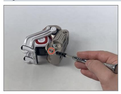
Remove the 5.5 mm screw on the right side of the front gold bumper using a JIS #1 screwdriver.
