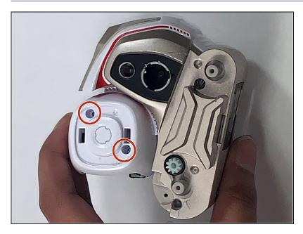
Remove the two 5.5 mm screws from the right side of the white head using a JIS #0 screwdriver.
