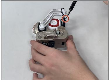
• Remove the 5.5 mm screw on the left side of the front gold bumper using a JIS #1 screwdriver.
