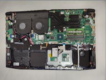
• Lift the battery up and out of the laptop.
