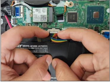
Disconnect the battery's motherboard connector with your fingers.
