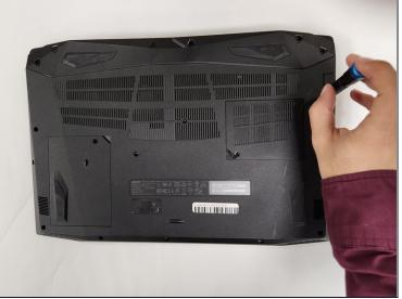
• Use the Phillips #0 screwdriver to unscrew the sixteen 9 mm screws holding the back cover in place.
