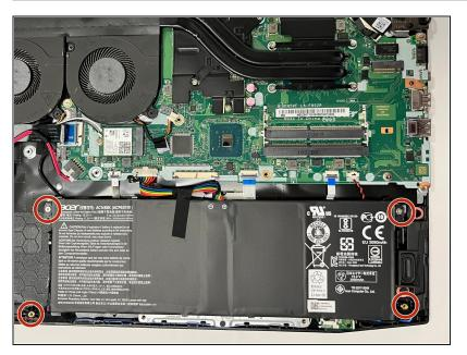
Use the Phillips #0 screwdriver to unscrew the four 9 mm screws holding the battery in place.
