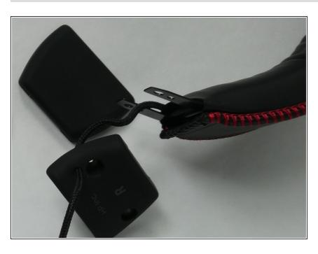
Remove the black plastic clips, freeing the metal sliding band inside.
