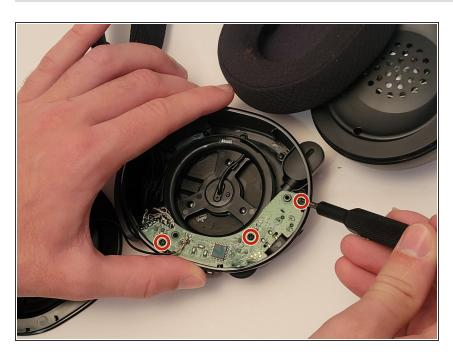
Use a Phillips #0 screwdriver to remove the three 5 mm screws.
