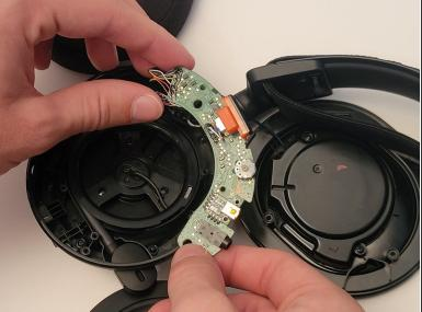
Remove the circuit board by pushing the scroll wheel out of the board and pulling it from the other side.
