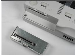
Remove the expansion bay by applying pressure to the small clip on the expansion bay while
