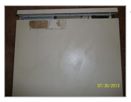
Using both hands on each side of the case, slide the top cover toward you. Lift it up off the computer.
