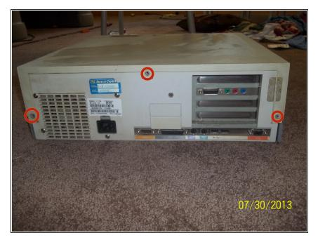
Remove the 3 Philips head screws from the back of the computer using your Philips screwdriver.
