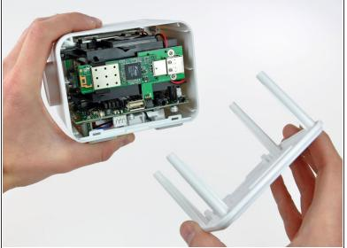
Remove the rear cover from the device.
