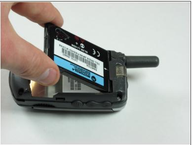
• Remove battery by grabbing it near the bottom and lifting out.
