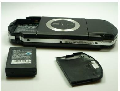
Using your finger, remove the battery upwards from the system as shown.
