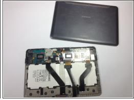
• Using the plastic opening tools, continue to carefully run along the right and bottom edge, and then lift the screen from the back panel.
