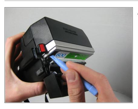
Using a plastic opening tool, rotate gear downward until jam is cleared.
