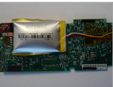
3. Remove battery by carefully detaching the connect wire that's connected to the circuit board.
