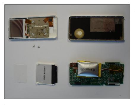
6. Finally you should have the ipod dismantelled and you should be able to put the ipod back together.
