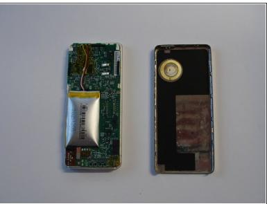
1. Using an ipod unclipping tool (which could be a knife or similar to it), unclip the outer casing by putting the tool into the connection point. This should pop the case off. Note that force will need to be used.
