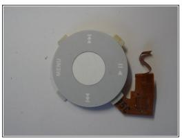
• 5. Removing the touchpad is easy and simple as there are layered parts on top of each other, just simply pull them off.
