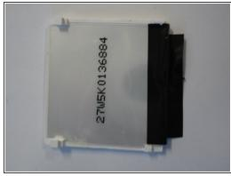
• 4. The screen has 3 different sections, each held down by glue so necessary force is needed. First remove the acrylic backing that supports the screen and then the main part of the screen. The last thing to remove is the paper-thin cover.
