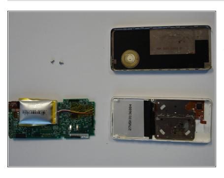
2. Remove the circuit board by unscrewing the 3 screws that hold it down. Note that specialised screwdrivers may need to be used.
