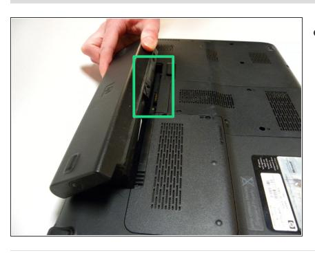
Place the new battery into the battery bay, making sure the connectors are lined up so the battery can click into place.
