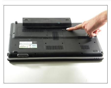
With the battery facing away from you, slide and hold the battery release latch to the left.
